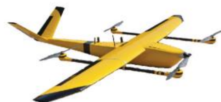
H20型垂直起降固定翼无人机 H20 Vertical Takeoff and Landing Fixed-wing UAV
