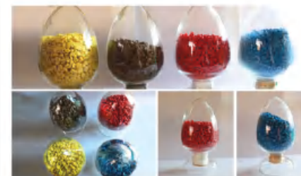
70°C绝缘级软聚氯乙烯塑料 70 Degree Insulation Grade Flexible PVC Plastic
